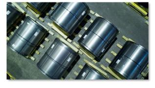
a form of cold rolling with slight compression and no lubrication. Temper rolling improves the surface quality of the steel. The final stage is processing. The sheets or coils are edge-trimmed, cut to length, and oil coating. As a structural and construction material, cold-rolled coils belong to widely used products. This necessitates their production in a wide range of sizes from various grades of carbon, low-alloy, and alloy steels.
